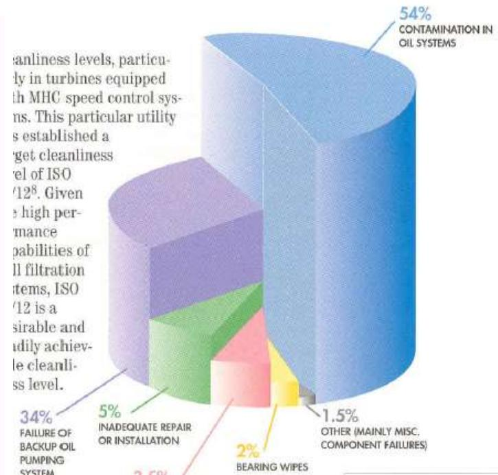
Lube Oil failures is the first cause of turbines unplanned outage (GE 1991)
